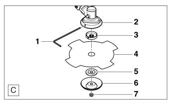
Unscrew the locknut (C/7) from the shaft by turning it clockwise. If necessary, block the angle gear (see below).
